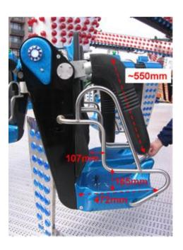
It can be seen that the original side restraint bars are retained and the new piece welded to it. This addition should be capable of withstanding the weight of the upper torso of a large male rider, an approximate sideways force of 150 kg during all phases of the ride.
