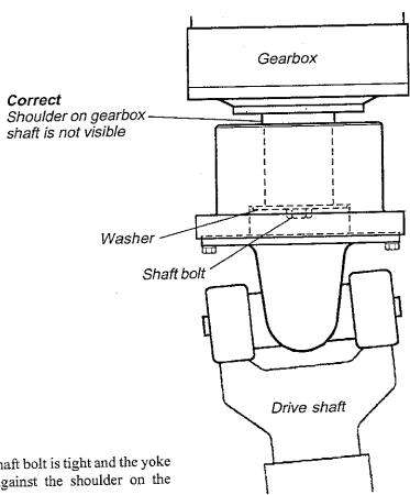
This condition indicates the shaft bolt is tight and the yoke adapter is properly seated against the shoulder on the gearbox shaft.
