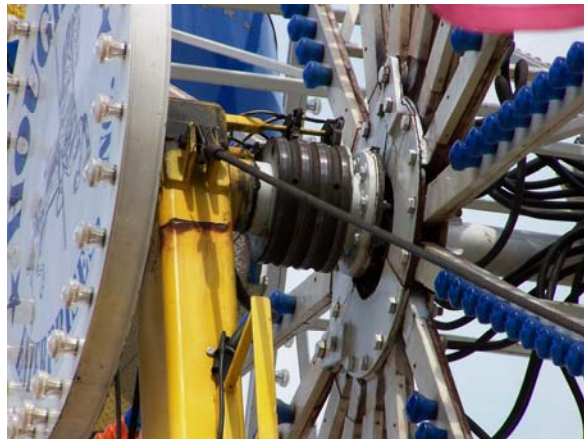
HUB WITH BROKEN AXLE
