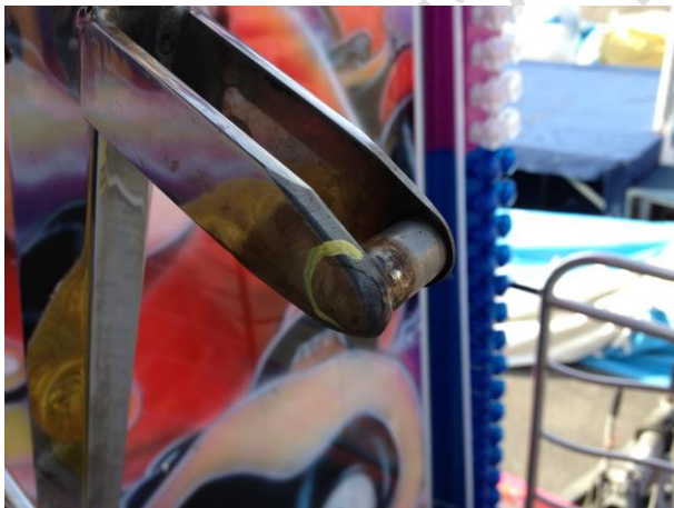
2) weld/ material defect found on lap bar lock
