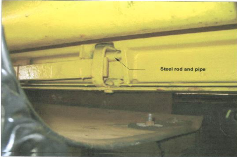
picture 1: Brake after modification
