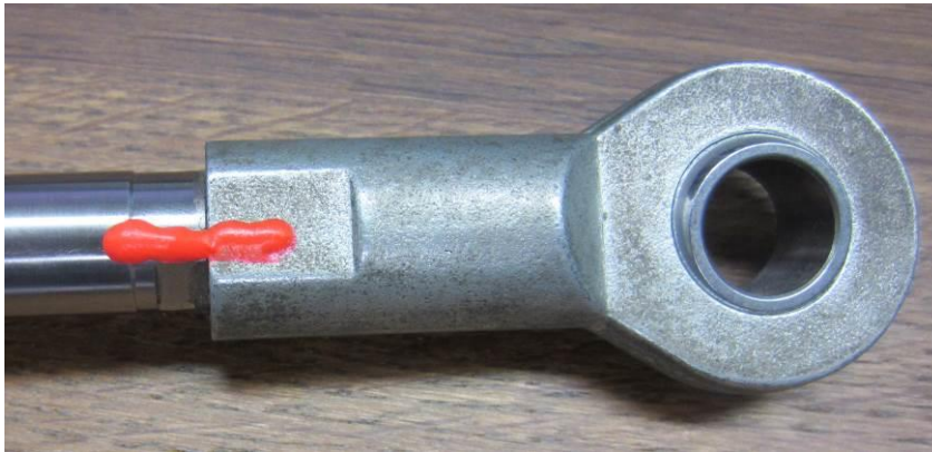
Figure 1: how to apply torque striping on the rod end.
