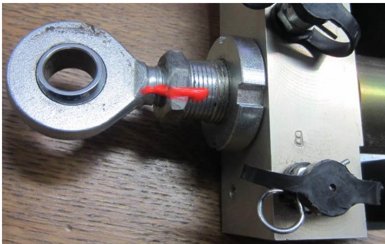
Figure 2: how to apply torque striping on the threaded screw assembly at the bottom.
