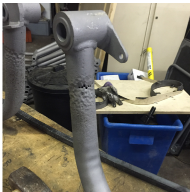
2) Showing corrosion of tube steel section.
