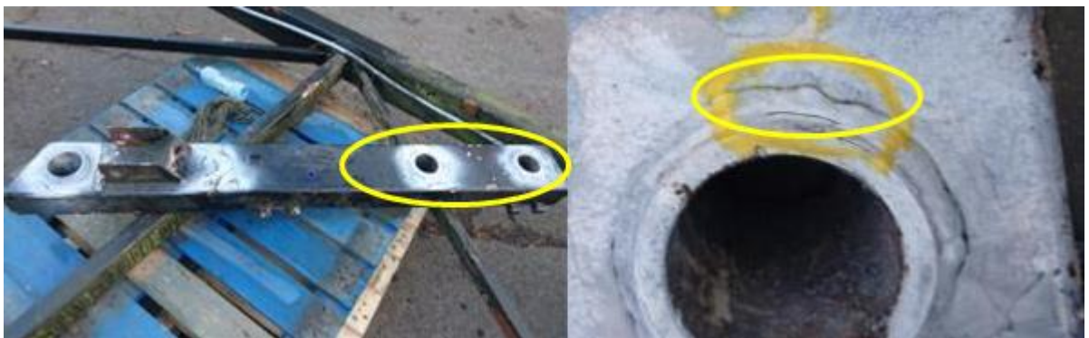
Intermediate lower A-Frame pin circular bore cracking. (visual & mpi)
