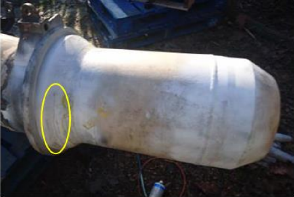
Main leg spigot cracking (visual, mpi & UT)
