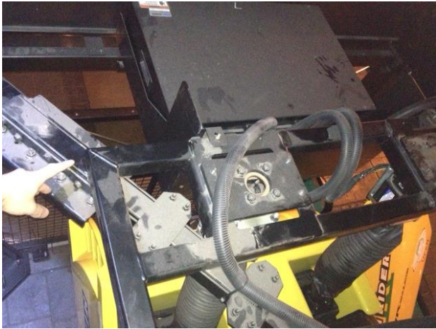
Main area of cracking, looking from the top of the frame. Cracks extend across the top of the 50 x 50 mm box section and down either side (possibly also underneath).
